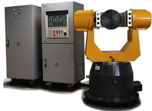
Slip ring assemblies featuring power rings and shielded signal rings permit electrical access to the UUT and allow to simulate continuous rotation. Beside the standard slip ring configuration, a wide variety of slip ring capsule designs and wiring schematics are available.
