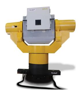
Slip ring assemblies featuring power rings and shielded signal rings permit electrical access to the UUT and allow to simulate continuous rotation. Beside the standard slip ring configuration, there is a wide variety of slip ring capsule designs and wiring schematics available.
